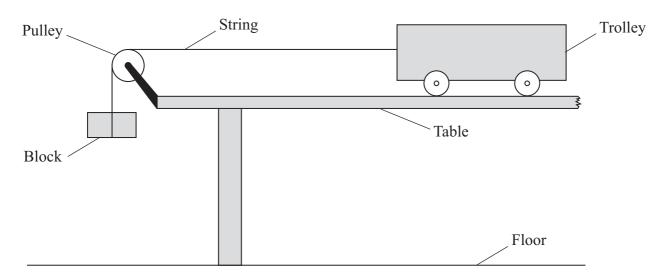
As the block falls it loses gravitational potential energy and the trolley and block together gain kinetic energy. The student is asked to find out what fraction of the gravitational potential energy becomes kinetic energy.
